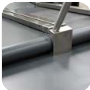
Low gap between conveyors eliminating the risk for the baggage to get stuck in transition
